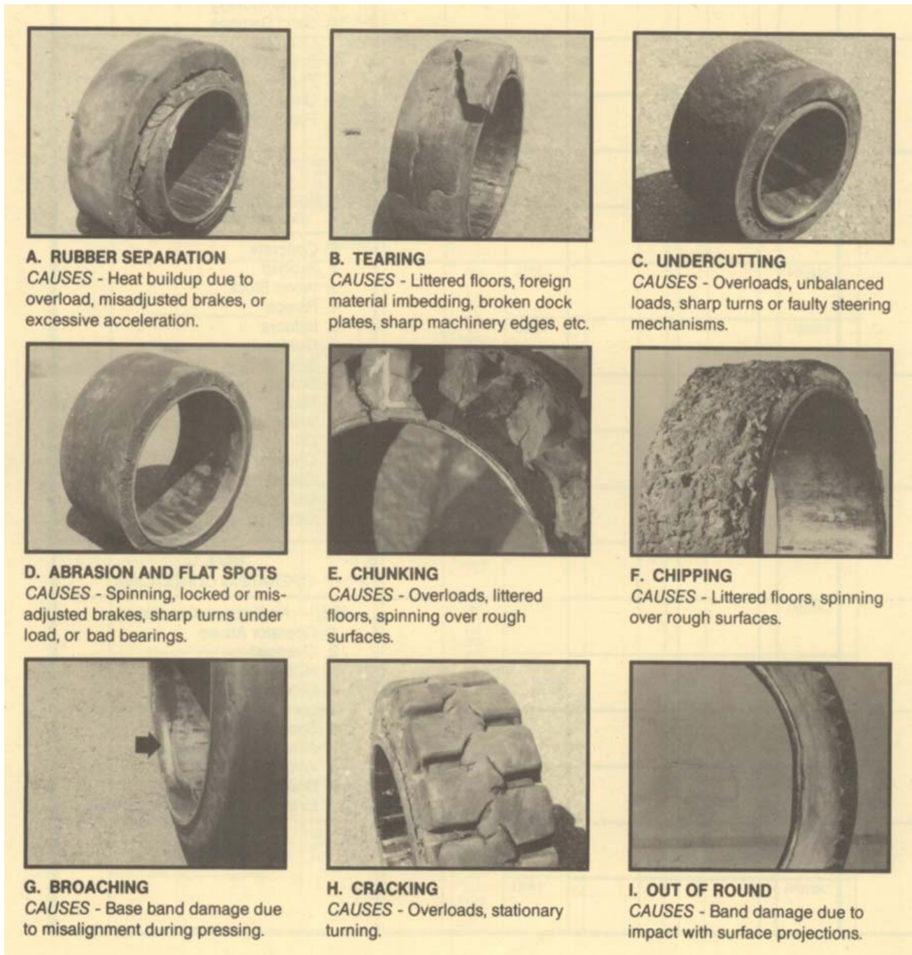
FIGURE 8-7. Solid Rubber Tire Defects
